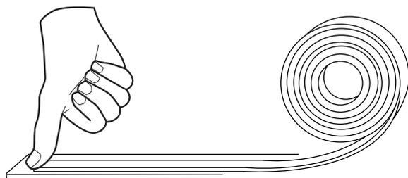
Make sure that the surface on which the tape will be applied is clean. Place the tape on the desired surface; apply moderate pressure for few seconds and release. (Keep in mind not pressing too much if there are electronic components on the other side of the PCB).
